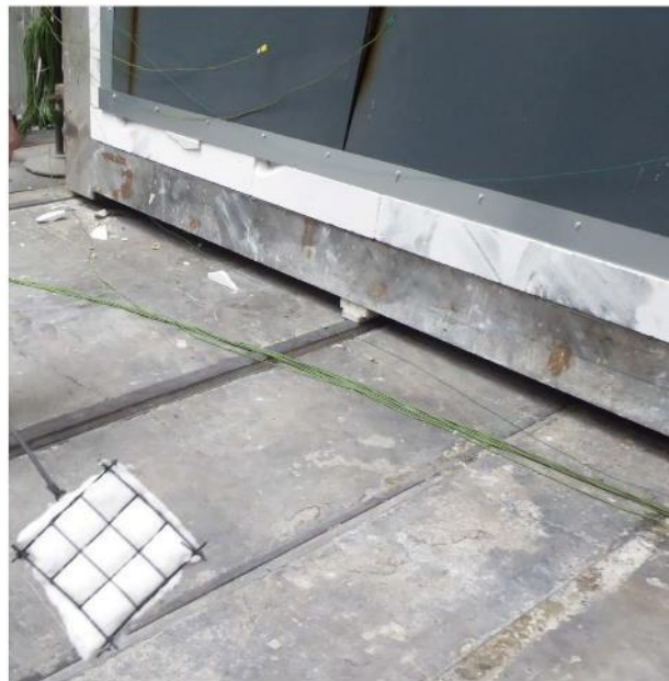
UF in 105 th minute of the test - cotton pad test - without integrity failure
