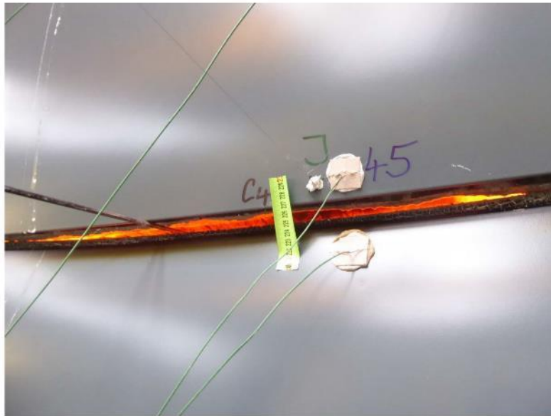
UF in 94 th minute of the test - 6 mm gap gauge can't pass through the specimen - without integrity failure
