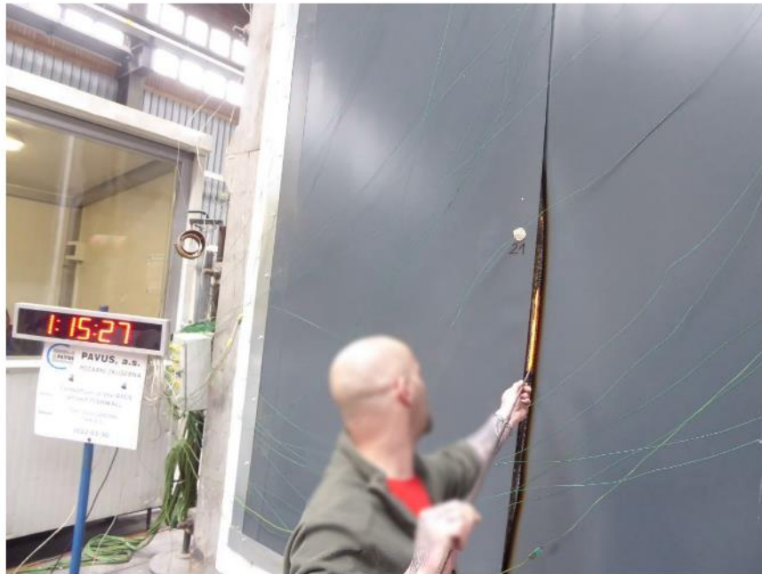
UF in 76 th minute of the test - 6 mm gap gauge can't pass through the specimen - without integrity failure
