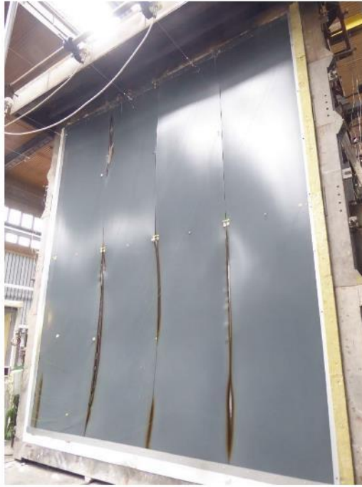
UF after 108 minutes - end of the test
