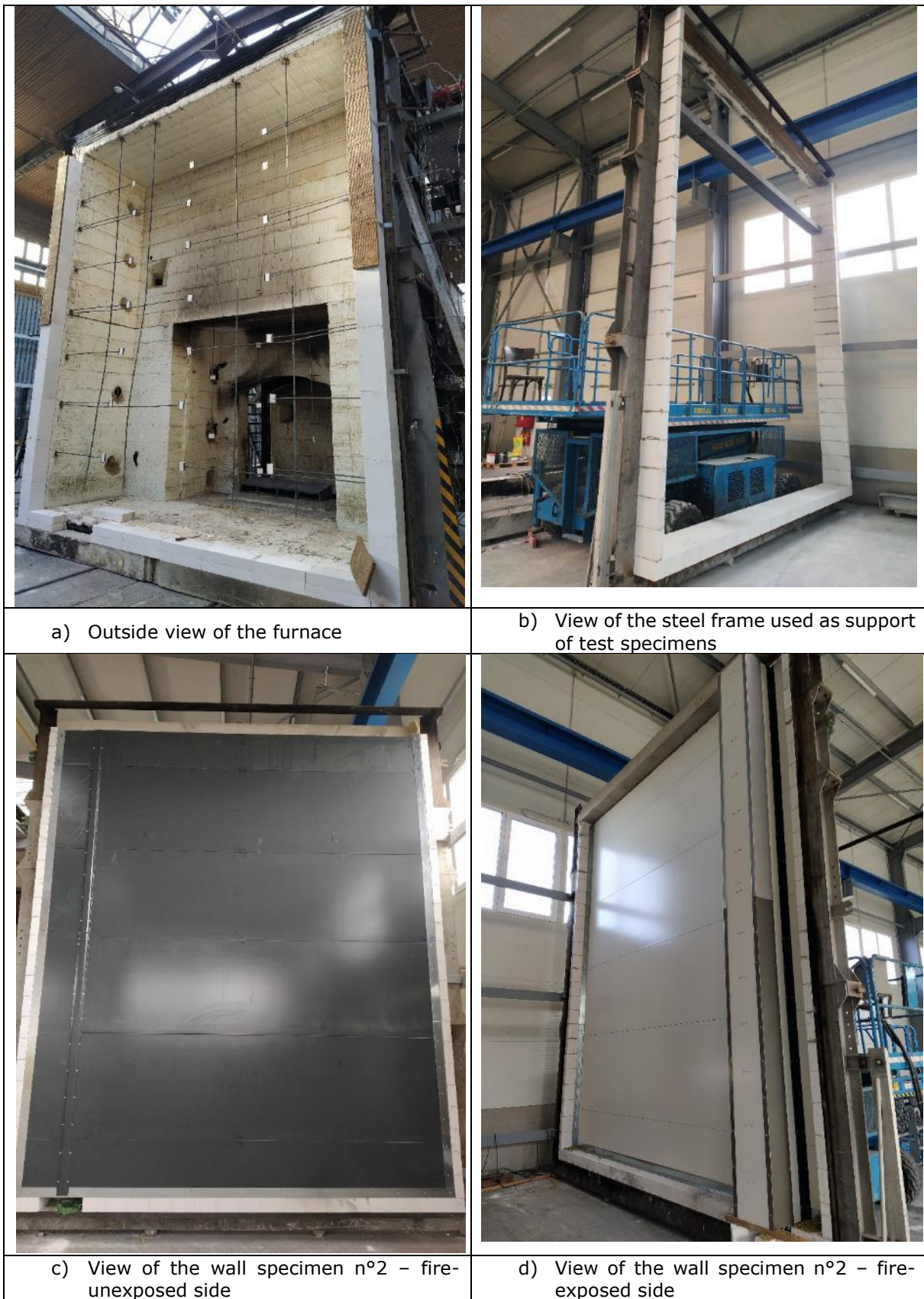
Figure 1: Views of the testing setup and test specimens
