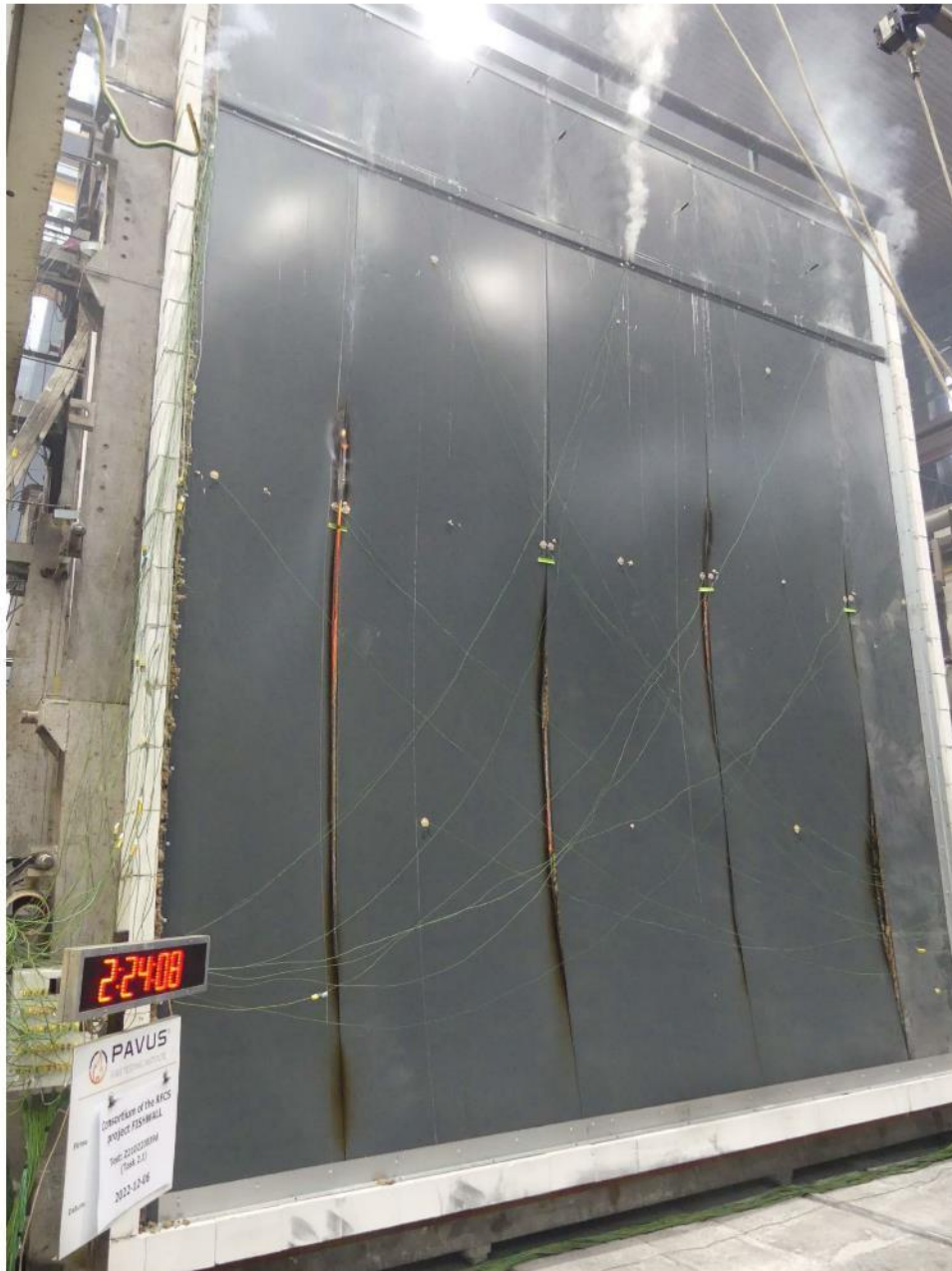
UF after 144 minutes - end of the test
