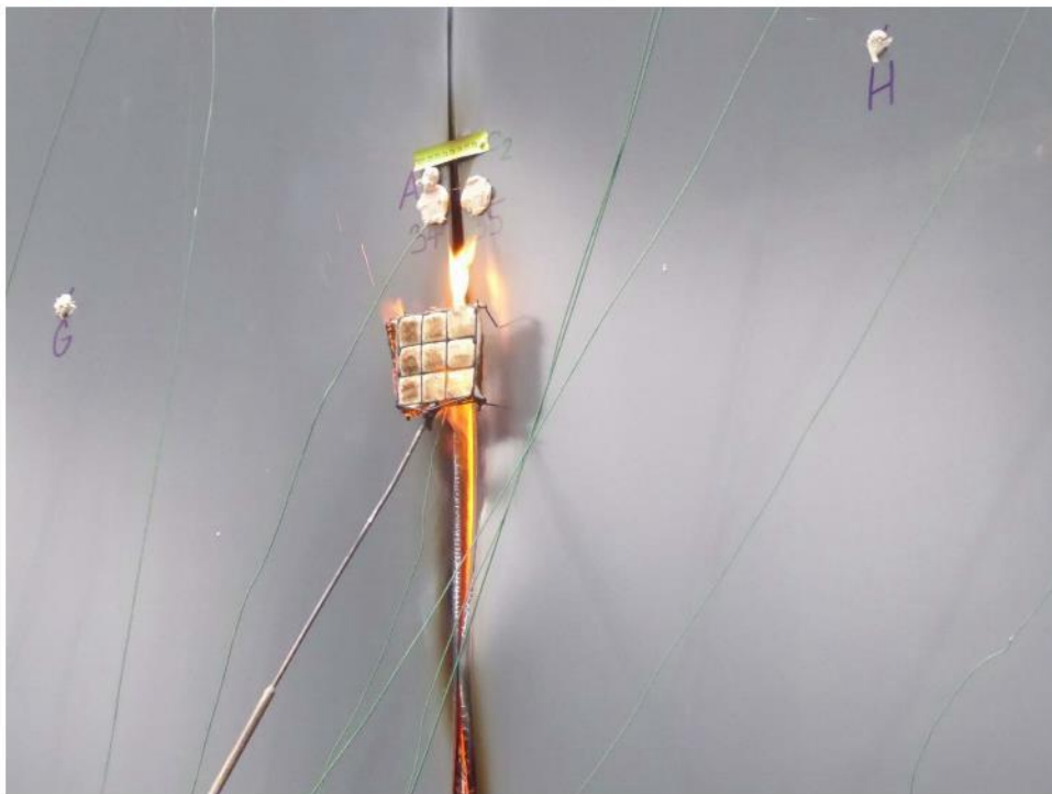
UF in 107 th minute of the test - cotton pad test - integrity failure
