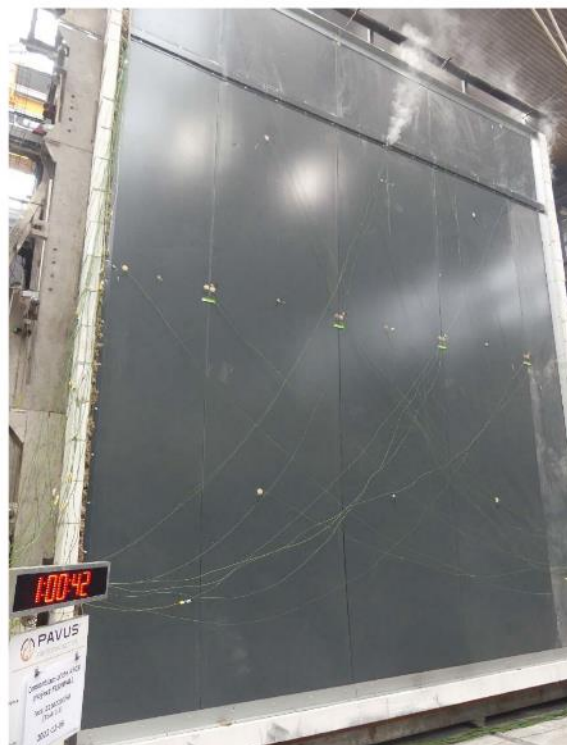
UF after 60 minutes of the test
