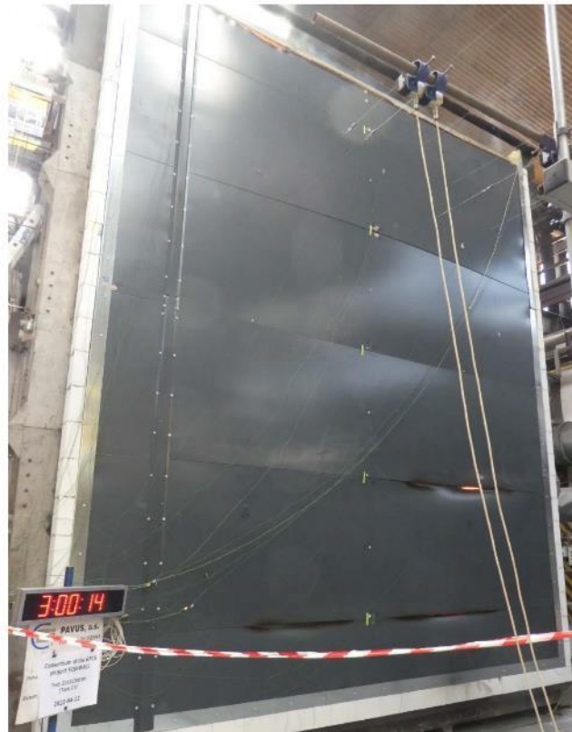
UF after 180 minutes - end of the test
