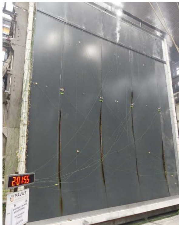
UF after 121 minutes of the test
