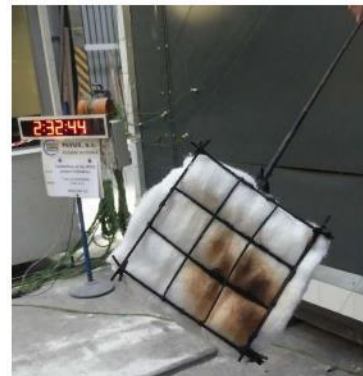
UF in 153 th minute of the test - cotton pad test - without integrity failure
