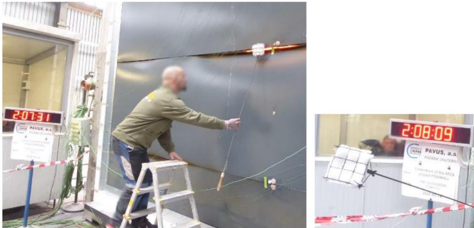
UF in 128 th minute of the test - cotton pad test - without integrity failure
