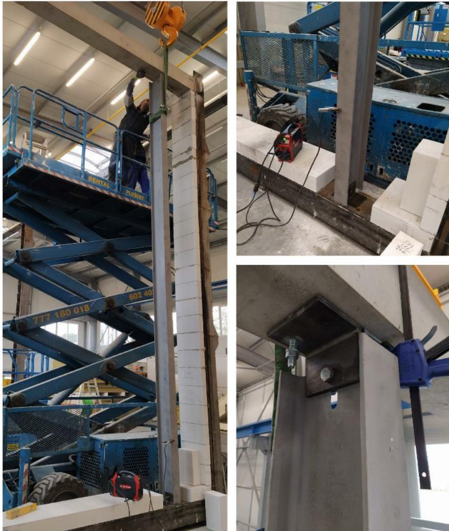
Assembly of the steel column
