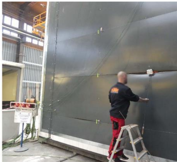
UF in 153 th minute of the test - cotton pad test - without integrity failure
