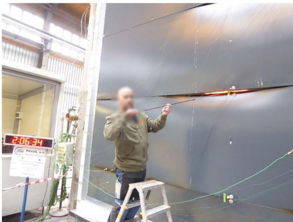
UF in 127 th minute of the test - 6 mm gap gauge passed through the specimen in distance longer than 150 mm along the gap - integrity failure
