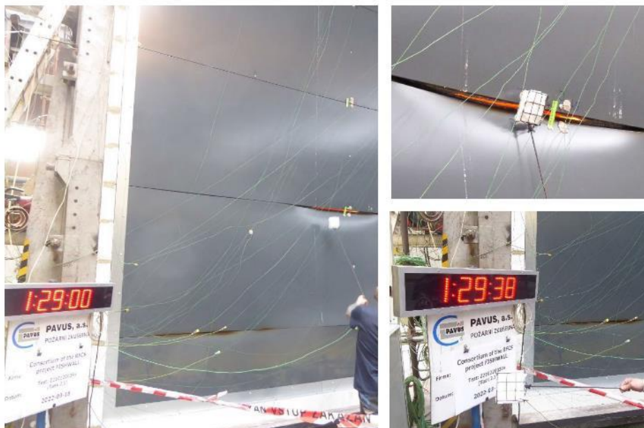
UF in 90 th minute of the test - cotton pad test - without integrity failure
