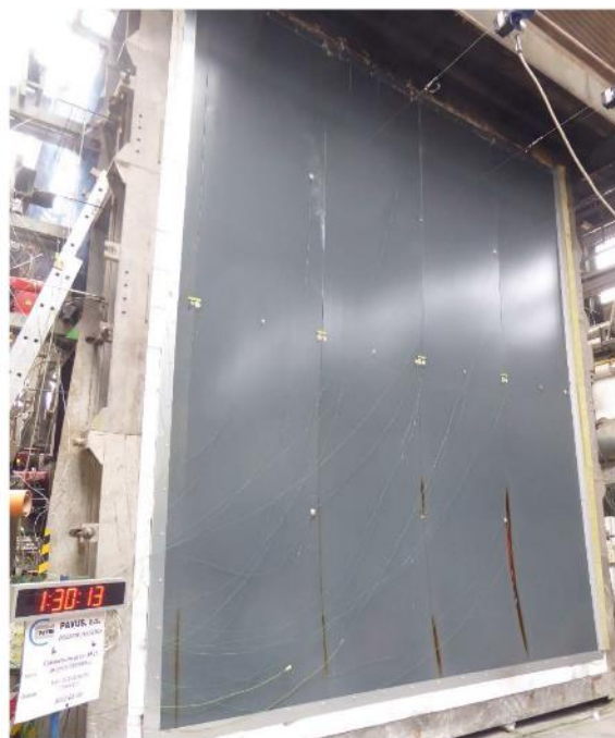
UF after 90 minutes of the test
