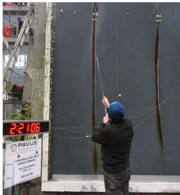
UF in 142 nd minute of the test - 6 mm gap gauge can't pass through the specimen - without integrity failure
